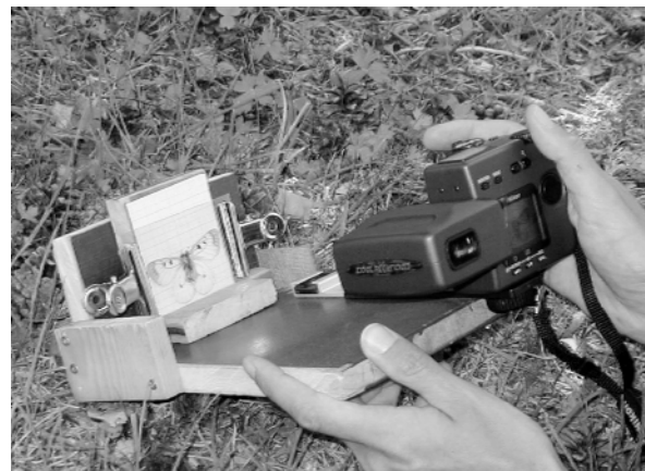
Fig. 1. The stand in the field, with a specimen of Parnassius mnemosyne being photographed.
